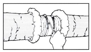
**3.** Pull jacket and insulation back over cores. Tape jackets together with at least 2 wraps of duct tape.
