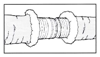
2. Tape cores together with at least 2 wraps of duct tape. Secure connection with 2 clamps placed over the taped core ends and past the beads.
