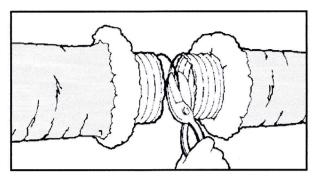
2. Slide at least 1" [25 mm] of core over fitting and past the bead. Seal core to collar with at least 2 wraps of duct tape. Secure connection with clamp placed over the core and tape and past the bead.
